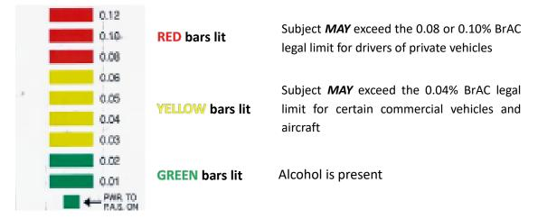
In some situations it is not practical to get the PAS sensor as close as 5–7 inches from the subject's mouth. The device can be used at greater distances, but readings will be lower. As a rule of thumb, one less bar will light up for every 2 inches beyond the optimum 5–7 inches. Using the PAS Flashlight at distances greater than 10 inches is not recommended for breath-alcohol sampling, because of the effect of drafts.
