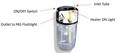
The lower (jar) portion is filled with a heated solution of water and alcohol, which simulates the blood running through the arteries in the lungs. The upper portion (the head space) is filled with a mixture of air and alcohol that simulates the air in the lungs that is in contact wit the blood across the cell membranes. Air flowing out of the outlet pipe simulates the expired air of a person who has been drinking.
